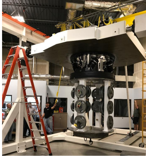
Figure 10: Proof load testing of the camera hexapod and rotator with a 2X payload mass at a 90 deg elevation angle
