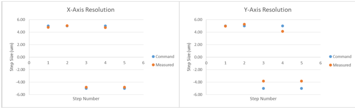
Figure 12: Resolution test results for X and Y-axes of camera hexapod
